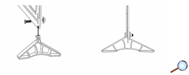
2. Slide stabilizer foot onto cargo divider panel at each corner, aligning the hole in the foot to the vertical slot in the panel.
