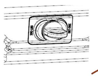
3. Prior to assembly, ensure tie downs are tightened and oriented horizontally.
