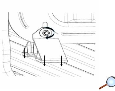
6. With cargo divider resting on top of the tie downs, push stabilizer foot down so that both legs rest flat against the pick up bed floor.
