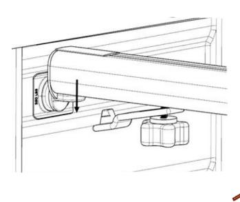
5. With the end caps pointed down and the protectant strips facing up, place the cargo divider on top of each of the opposing tie down loops.
