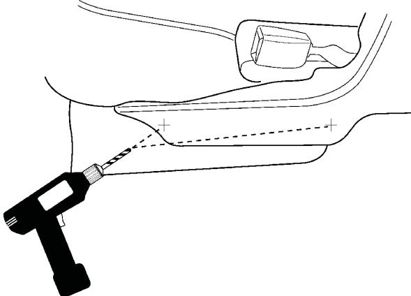
2. With seat in upright position, and using a 1/8" drill bit with a 1/4" drill stop, carefully drill the marked areas on the seat's plastic side panels. Be sure to not pass through the seat's plastic side panels more than 1/4" in depth. Then enlarge the pilot holes using a 5/16" drill bit with a 1/4" drill stop. Vacuum plastic drill shavings when finished.
