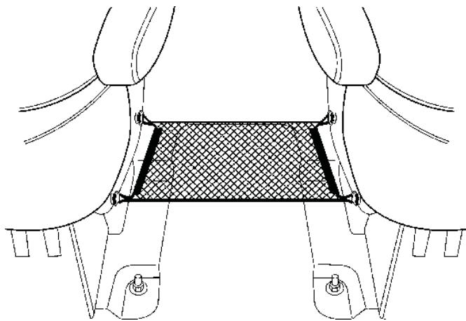
4. With seat in upright position, this is what your finished installed net assembly should look like. Please note to detach the net assembly during fold and tumble operation of the seat.
