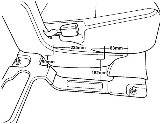
1. With seat in upright position, measure and mark the right-side plastic seat panel of the drivers-side 2nd row seat in the following locations for drilling. Repeat for step for passengers side 2nd row seat left-side plastic seat panel.
