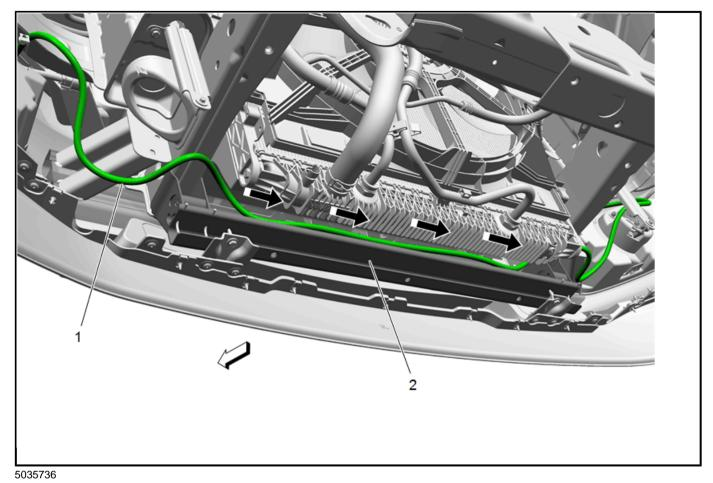
2. Route the wiring harness (1) across the base of the radiator and loosely tie strap to the cross vehicle beam (2).
