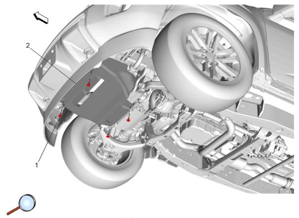
7. Install the underbody splash shield (2). Refer to Vehicle Service Manual.
