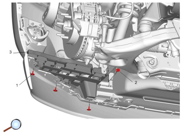
2. Remove the front bumper intermediate filler (3). Refer to Vehicle Service Manual.
