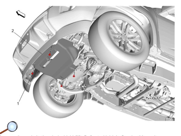
3. Remove the underbody splash shield (2). Refer to Vehicle Service Manual.
