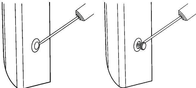
3. Attach the cords to the sidewall attachment anchors as shown. Attach the net hooks to the cord loops as shown.
