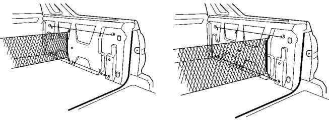
5. The net can be placed along the Cargo Bed Side walls by attaching the net hooks to the sidewall cargo tie-down D-rings.
