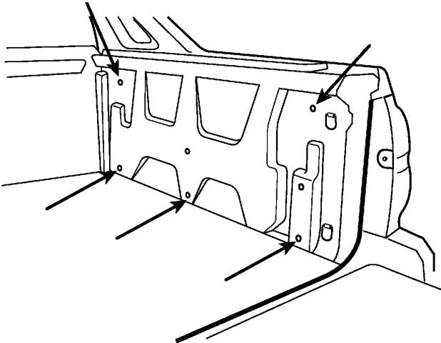
2. Remove each Cargo Bed sidewall trim, push pin plug as shown and replace with the mushroom attachment anchors provided with the net kit. Repeat for other side of Cargo Bed sidewall.
