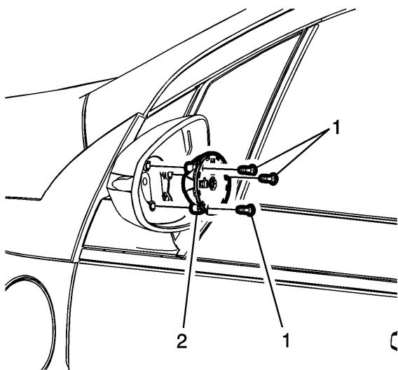
7. Remove the outside rearview mirror inner actuator screws (1). Retain screws for reassembly.
