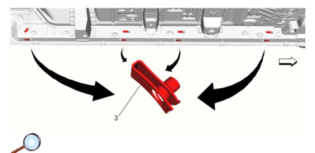
1. Install the eight - U-nuts (3) into existing holes on rocker inner panel. Refer to graphic for locations and orientation of U-nuts. Install the U-nuts with the threads inside the rocker inner panel.
