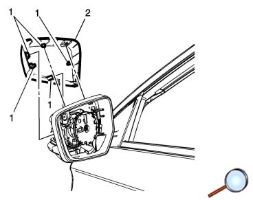
1. Align the mirror housing cover (2) with the base of the outside mirror housing assembly, push forward until the housing cover is fully seated into the outside rearview mirror base.
