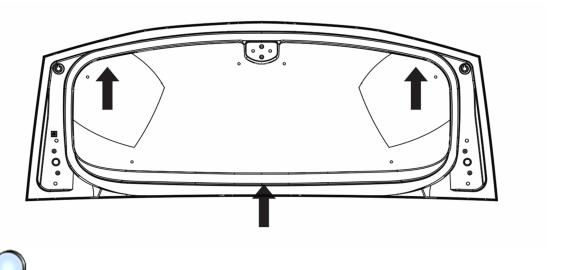
8. Firmly press the cover at the bottom center and the top corners to attach the Velcro®.
