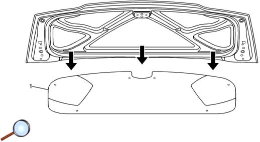
3. Remove the liner (1) from the frame.
