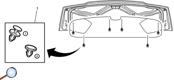
7. Insert the push-pins (1) (unlocked) into the holes, then lock them in place by pushing down on the top.
