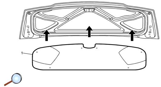
6. Press the liner (1) back onto the frame without pressing down onto the Velcro®.
