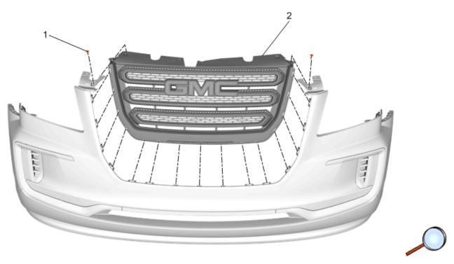
**Note:** Each individual front bumper fascia tab must be secure to each slot in the front grille prior to reassembly of the fascia to the vehicle.
