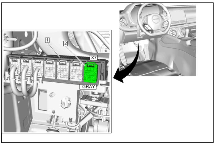
11. Locate the BCM (1) on the driver side of the vehicle, under the I/P. Disconnect BCM connector (2) X7 gray.
