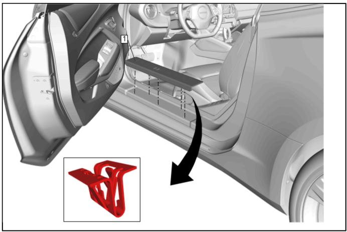
3. Remove the left and right non-lit front door sill plates. Refer to Vehicle Service Manual.
