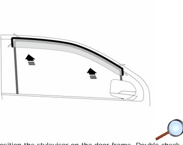
4. Position the stylevisor on the door frame. Double check the positioning of the stylevisor following the dimensions shown in step 1, the apply light pressure to the tape areas.
