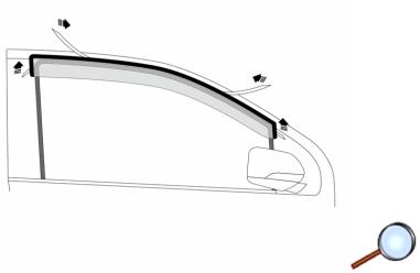
5. Slowly peel the remaining protective tape liner away by pulling on the exposed ends of liner, and apply firm pressure around the attachment areas.
