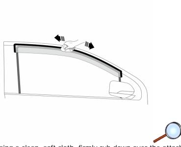
6. Using a clean, soft cloth, firmly rub down over the attachment areas 4 times to ensure maximum adhesion.
