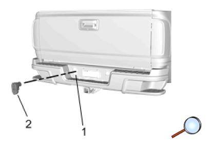
1. Remove the cap on the left side of rear bumper (1) where trailer connector will be installed.
