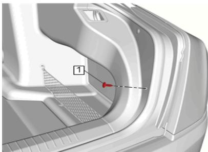
2. Displace soft trunk trim to expose metal bracket behind panel as shown in Figure 2.
