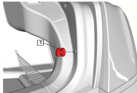
6. Attach convenience net upper loops around T shaped retainers as shown in Figure 5 (both sides of vehicle).
