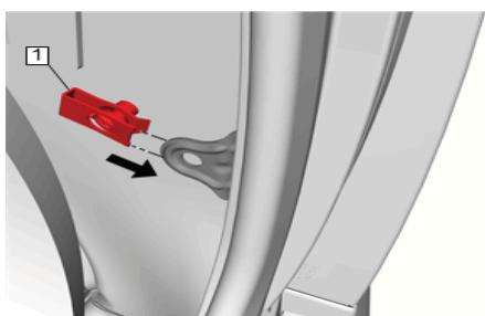
4. Retrun soft trunk trim to installed position, align holes and screw T shaped retainer into J-Nut as shown in Figure 4.
