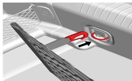
7. Attach convenience net upper loops around T shaped retainers as shown in Figure 6 (both sides of vehicle).
