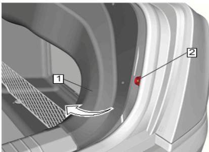
3. Insert J-Nut around the exposed metal bracket as shown in Figure 3.
