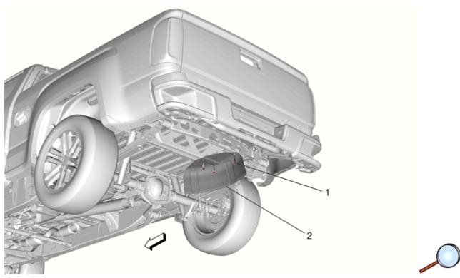
9.2. After removing the spare tire from under the pickup box, remove the 3 plastic retainers (1) that retain the spare tire heat shield (2), and discard the heat shield.
