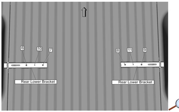
4.2. Set the Spare Tire Carrier Assembly (item 1) aside. Use the Rear Lower Carrier Bracket (item 3), flat side down with slots outboard and centered on the markings for Holes (6 & 7), to mark the center of Hole (10), as shown. Repeat step to mark the center of Hole (11).
