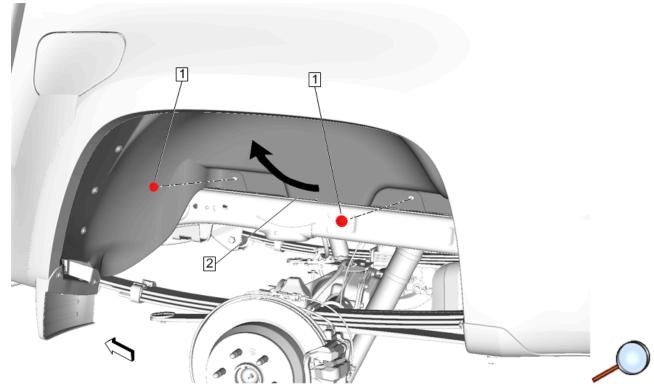
6.1. The LH and RH rear wheel liners will need to be pulled upward temporarily to allow for installation of the Rear Lower Carrier Brackets (item 3) into the pick-up box center cross sill. Locate the rear wheel liner (2) at either side of the vehicle and remove the two screws (1) shown below to allow access to the cross sill.
