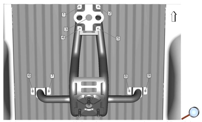
4.1. With the Spare Tire Carrier Assembly (item 1) in position, use a marker to carefully mark the center of Holes (1-9), as shown, on the pick-up box floor. When the holes are marked and verified to be centered with the Spare Tire Carrier Assembly (item 1), use a center punch to mark each center. If the vehicle is equipped with a spray-in bed liner, a white paint pen or alternative can be used to mark the hole centers.
