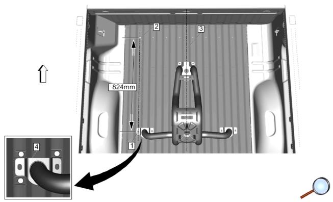
3. Spare tire carrier assembly – Position for EXTENDED CAB and CREW CAB Long Box (6'-2") Vehicles: Locate the 13.1mm diameter gage hole (2) in the front, left-hand corner of the pick-up box floor. Center (3) the Spare Tire Carrier Assembly (item 1) cross-car on the pick-up box floor. Position the assembly so that the fore/aft distance between the pick-up box gage hole center (2) and rear left Spare Tire Carrier Assembly attachment slot center (1) are 824mm.
