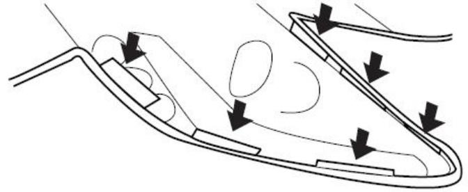
4. Attach the J-clips to the edges of the wheel wells.
