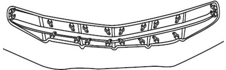
6. Attach the J-clips located on the bottom side of the mask to the underside of the car.
