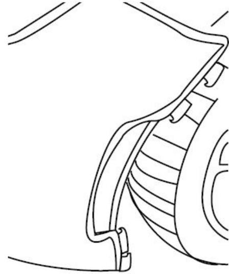
5. Attach the hooks to the edge of the grille opening.
