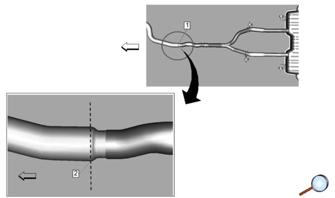
2. **Stock Exhaust Cut Location:** Raise the vehicle so that the center and rear section (1) of the factory exhaust can be reached. Cut the exhaust at the tangent point (2).
