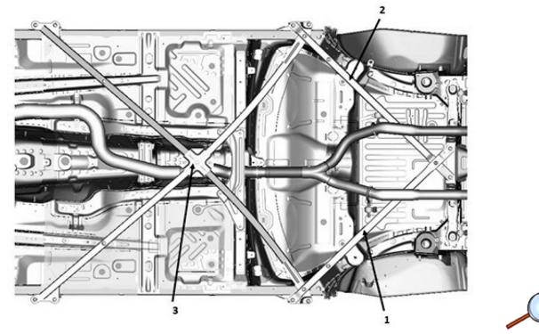
1. **Brace Removal:** For convertible vehicles, it is recommended that you remove the underbody bracing before replacing the accessory exhaust. Remove the braces in the order shown. Retain all fasteners for re-installation.
