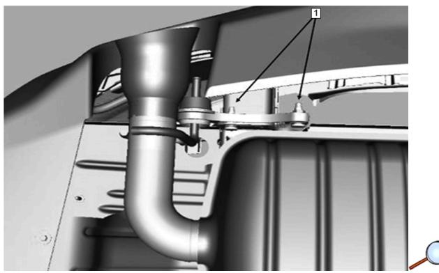
3. **Rear support bracket (LH shown, RH similar):** Remove the factory muffler from the hangers. Unbolt and retain the nuts (1) from the support brackets near both tailpipes at the rear of the vehicle and remove the support brackets from both sides as shown.
