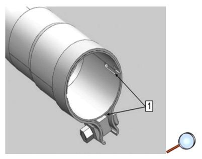
**Note:** Make sure two areas indicated (1) do not overlap when tightening. 11. Check orientation of all clamps. Notch (1) on pipes should not align with open area of band clamp.
