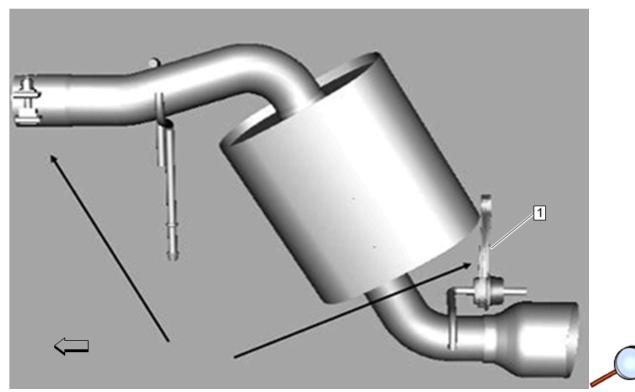
7. **Pre-installed Hardware on muffler:** Install a hanger over the end of one of the new mufflers, and install respective rear support bracket (1) onto muffler as shown.
