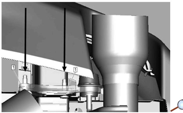
10. **Support bracket nut locations:** Once tip is aligned fore/aft, tighten two nuts (1) on rear support bracket as shown. Torque nuts to 40 Nm (30 lb ft). Repeat for opposite side.
