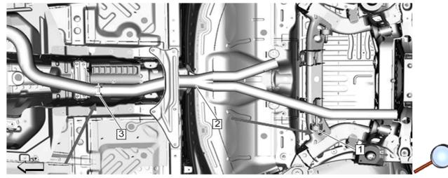
5. **Y-Pipe Installation:** Install Y-pipe (2) onto stock section. Loosely install clamp (3) and seat hanger into rubber grommet (1). Do not tighten clamp.
