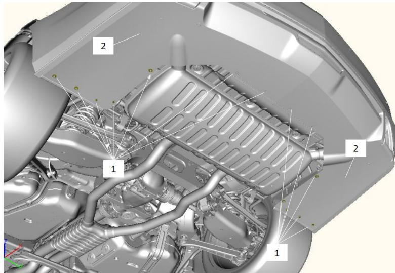
1. Beginning at the rear of the vehicle, remove the 14 bolts (1) from the lower fascia (2). The lower fascia cannot be completely removed but it will flex enough to allow removal of the factory exhaust.
