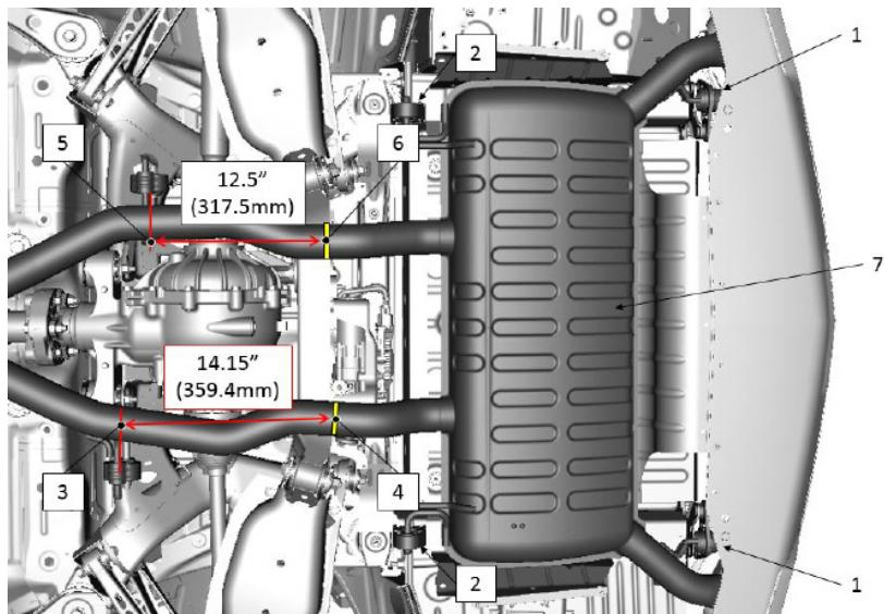
2. The passenger and driver side exhaust pipes pass under the subframe just behind the differential. Mark the center of the passenger side exhaust pipe where it intersects the rear edge of the hanger (3) and make another mark 14.15" to the rear of the vehicle to identify the center of the cut line (4) as shown in the picture above. Mark the cut line so it is perpendicular to the pipe.
