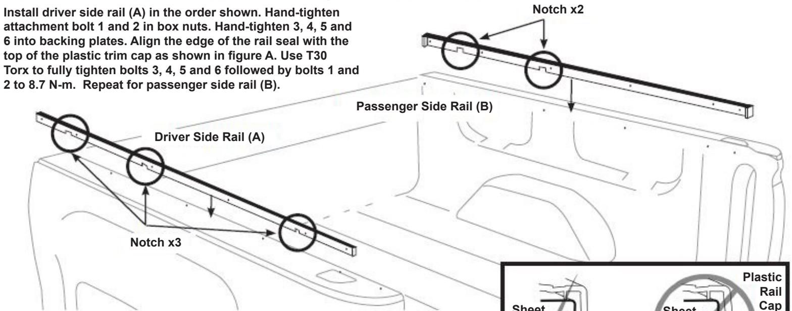
Backing plates are installed on the back side of the sheet metal.
