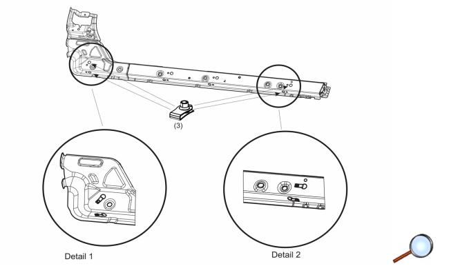
1. Install U-nuts (Item 3) onto existing holes in inner rocker panel. Refer to graphic (detail #1 and 2) for locations and orientation of U-nuts . Install U-nuts with the threads oriented so that they are inside of the inner rocker panel.
