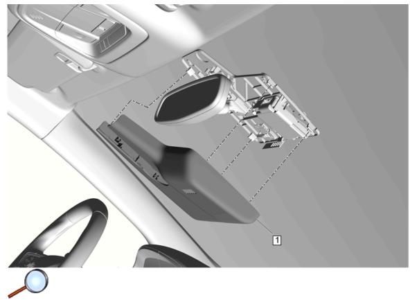
3. Carefully position the bracket lower cover (1) to the window engaging the retainers.
