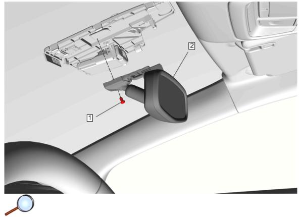
1. Position the Accessory Mirror (2) in the full upward position to the rearview mirror button and slide downward.
