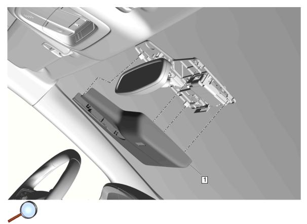
1. Using a plastic trim tool, carefully pry downward on the sides of the bracket lower cover (1) to release from the window.
