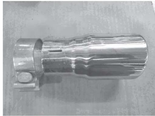
6. Place the exhaust tip assembly over the cut exhaust pipe until it aligns with the second exhaust measurement mark.
