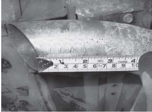
2. Place the exhaust tip clamp on the exhaust tip with the nut facing down.
