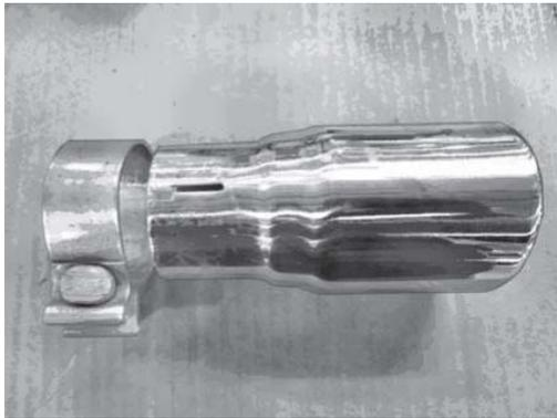
3. Place the exhaust tip assembly over the stock exhaust pipe until it aligns with the exhaust measurement mark.
