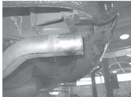
7. Align the exhaust tip so the drain hole is facing down.
