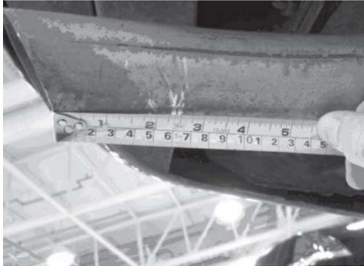
3. Using a reciprocation saw or a hacksaw cut the exhaust pipe squarely at the 2.25 (6.0 cm) mark.
