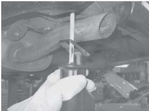
5. Place the exhaust tip clamp on the exhaust tip with the nut facing down.
