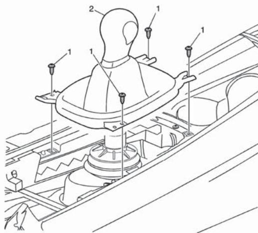
Next remove the 4 fasteners that hold the shifter assembly to the floor using a 10mm socket.
