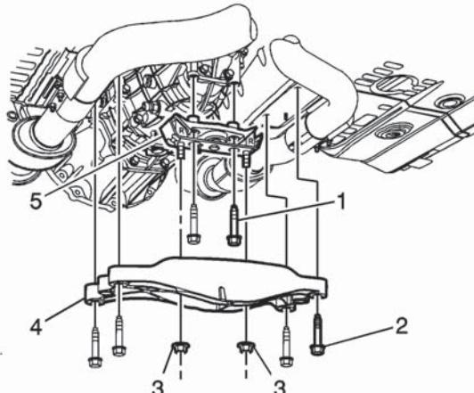
Lower the transmission down to gain access to the shifter assembly on top of the transmission.
