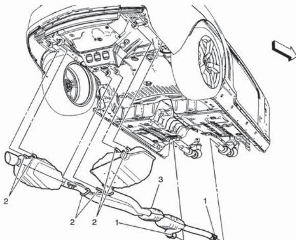
Remove exhaust heat shield to gain access to the driveshaft center bearing assembly.
