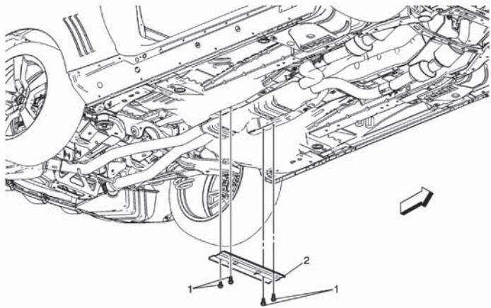
Loosen clamps at rear of catalytic converters and slide exhaust system rearward to disconnect from front pipes. (Exhaust does not have to be completely removed from vehicle as shown but may be helpful to remove it completely if not using a hoist).
