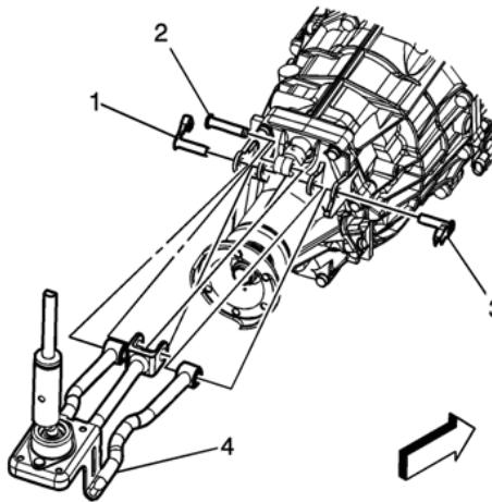
Raise transmission assembly back into position and at the same time position shifter into floor in the proper location. Reinstall transmission cross member to body bolts and torque to 58 N·m (43 lb-ft).
