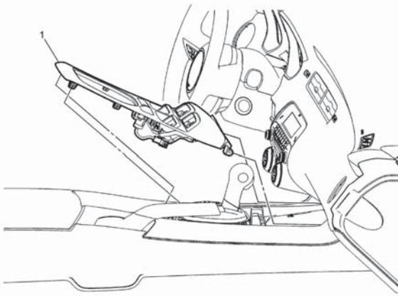
Remove the transmission control lever knob and boot assembly as shown below.
