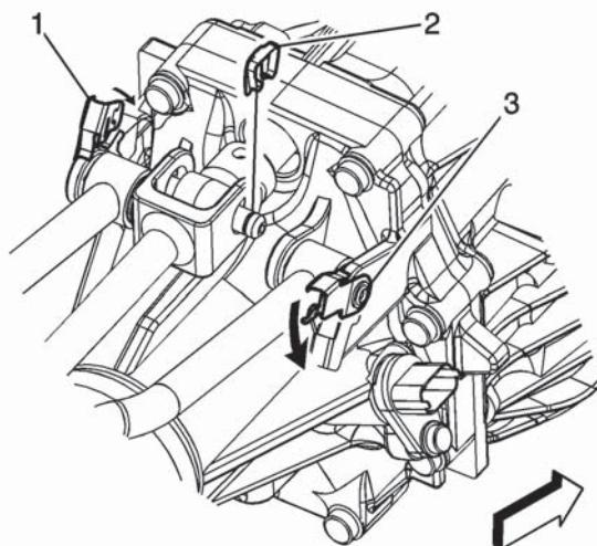
Using a flat-blade tool, release the center shift control rod pin retainer (2). (see above)
