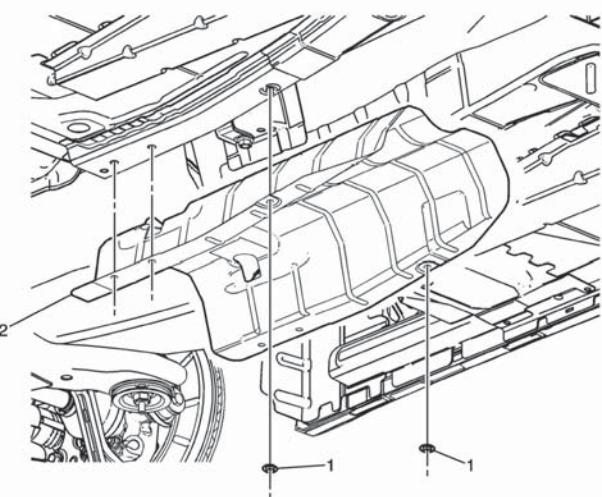
Remove the drive shaft center support bolts (2) and lower the center of the driveshaft.
