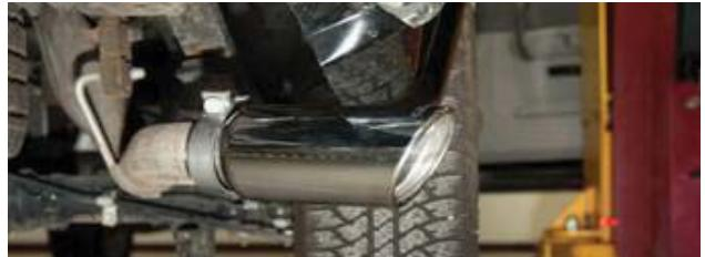
4. Tighten the clamp securing the tip to 32-35 ft. lbs.
