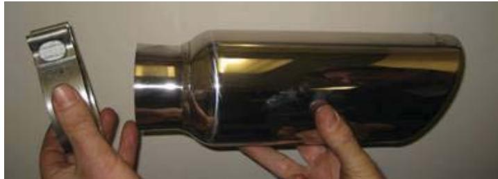
2. Measure from exhaust pipe outlet edge (bottom side) 8 inches inboard along pipe axis. Mark the pipe at the 8 inch dimension. Clean the end of the tube to facilitate a good tight fit.
