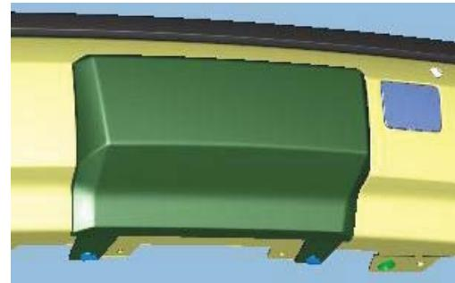
2. Mark and drill 6 holes for rivets.
