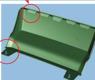
3. Secure the attachment bracket to fascia by using the 6 rivets.
