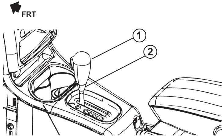
2. Set the shifter in neutral and engage the park brake. Pull the shifter sleeve or boot down to expose the set screw.
