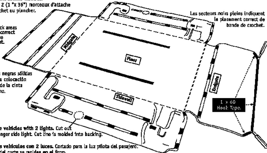
**3** Lay midgate down and lay BedRug in vehicle. Align for best fit by using cargo hook and cargo light openings for reference.
