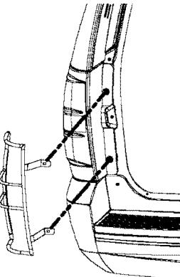
3. Insert new screws, provided in kit, through the tail lamp guard bracket holes, the tail lamp mounting holes and into inner vehicle mount. Apply pressure on the two brackets to ensure the brackets contact the side of the tail lamp. Tighten screws with screwdriver.
