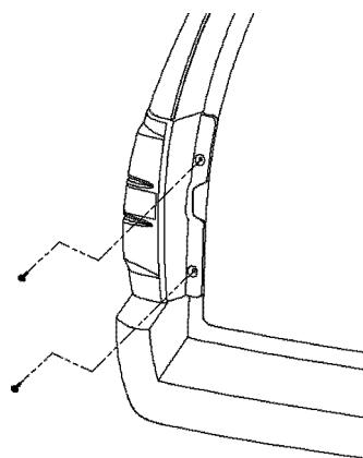
2. Position tail lamp guard over tail lamp. Align mounting holes in guard with holes in tail lamp.
