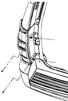
4. While applying outward pressure on tail lamp guard at lift gate side – to rotate tail lamp guard into the proper position - remove adhesive protector by pulling down on tape leader parallel to tape surface. Then, to adhere tape, apply pressure (30 PSI) inboard to tail lamp guard (over the tape) for 1 minute . Repeat steps for other side of vehicle.
