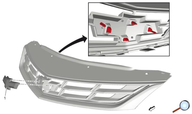
5. Remove the front emblem (1) by disconnecting the retaining tabs on the backside.
