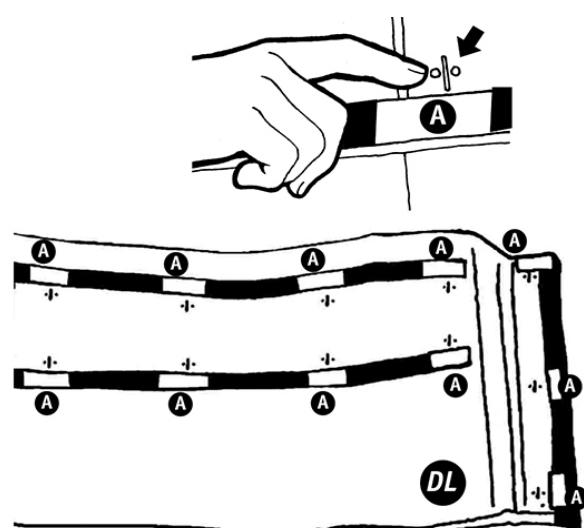
**4** Apply 1" x 63.5" (C1) hook tape to top of front panel (1).
