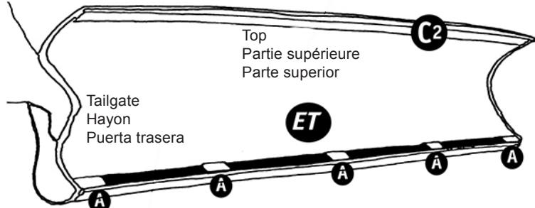
**6** Important: Make sure that Bed Rug is pushed completely forward and fits exactly in corners. Failure to locate liner properly may cause Bed Rug floor to bow when tailgate is closed.
