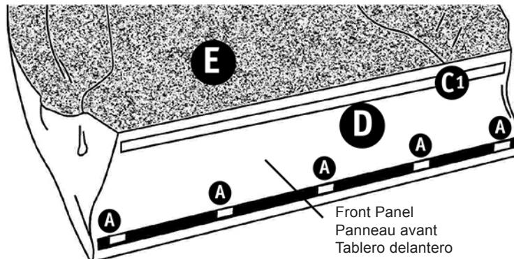
**5** Apply 1" x 60" (C2) hook tape to top (2) of tail gate.
