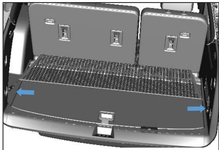
The hooks connect to the lower D rings on each side of the vehicle.
