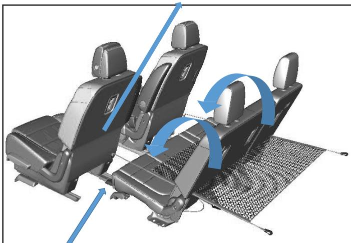
The hooks connect to the seat headrest post when the third row seat is folded down. The hooks should go on the outer post on both the driver and passenger side.
