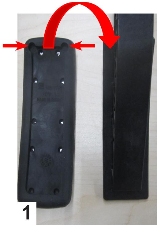
1. Ensure orientation of pedal is correct. NOTE: Top of pedal pad has circle cut corners.
