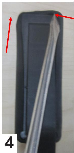
3. Rotate the pedal and using a flat blade screwdriver, carefully work along the edges of the pad.
