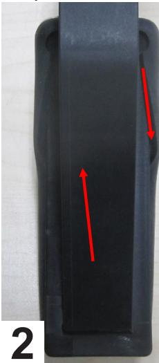
2. Attach top edge of pedal pad to pedal.
