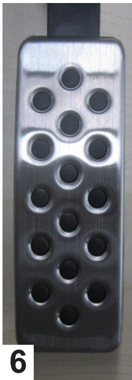
5. Inspect the pedal to ensure all edges are fully seated.
