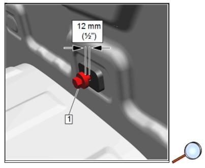
4. While pulling back on the hex bolt (1) 10-B, thread the bolt until approximately 12 mm (1/2") of thread is exposed.
