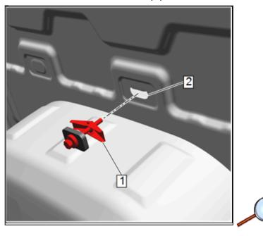
2. Insert the toggle assembly (1) item 10 in kit contents into the truck bed center hole (2).
