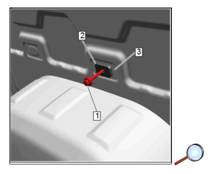
3. Pull back on the hex bolt (1) 10-B in kit contents and slide the rubber spacer (2) item 10-A in kit contents tight against the truck bed (3).
