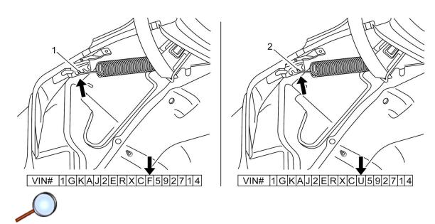
25. Remove the (Solid Black or Brown Stripe) factory installed deck-lid spring and replace with new (Dashed Brown Stripe) spring. Refer to Rear Compartment Lid Hinge Spring Replacement.
