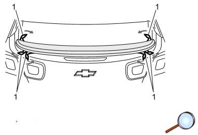
20. Remove tape liner by using the pull tabs (1).
