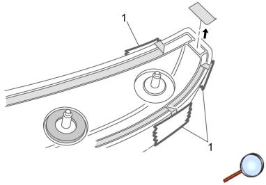
18. Fold the tape liner pull tabs onto the Spoiler surface and apply masking tape (1) to ensure that the pull tabs are accessible. Remove small piece of tape liner at either end of the spoiler.
