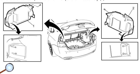
7. Reposition the left (1) and right (2) side rear compartment side trim panels enough to gain access to the left and right rear compartment lid hinge springs.
