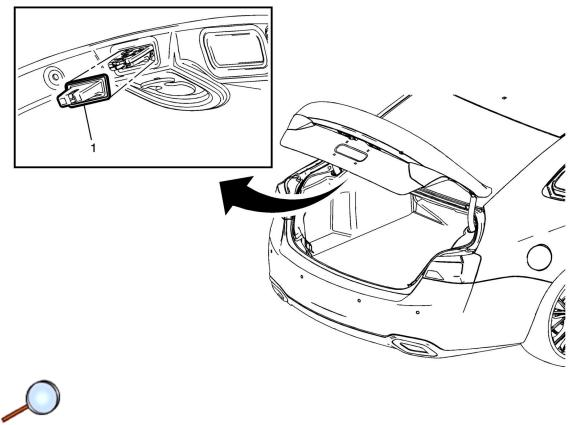
Using a small flat-bladed tool, pull and release the rear compartment cover (1).
