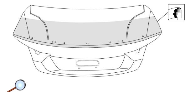
17. Using alcohol wipes, clean area where spoiler will be installed.
