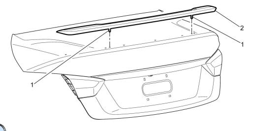
19. Carefully install the rear spoiler (2) by inserting the studs (1) into the holes in the trunk lid. Before allowing the plastic retainers to engage or tape to contact the trunk lid, make sure the spoiler is centered. Once this is confirmed push down and engage studs into plastic retainers.
