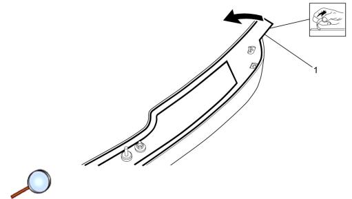
18. Remove tape liner (1) by using the pull tabs.
