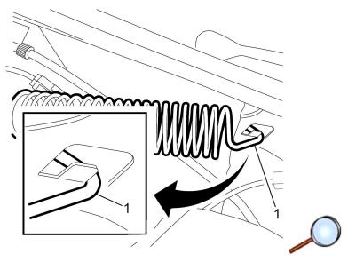
Warning: When a hood hold open device is being removed or installed, provide alternate support to avoid the possibility of damage to the vehicle or personal injury.
