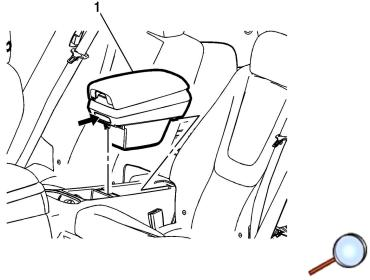
1. Push the lower bin button and lift the rear console (1) upward and forward to release it from the rear bracket.
