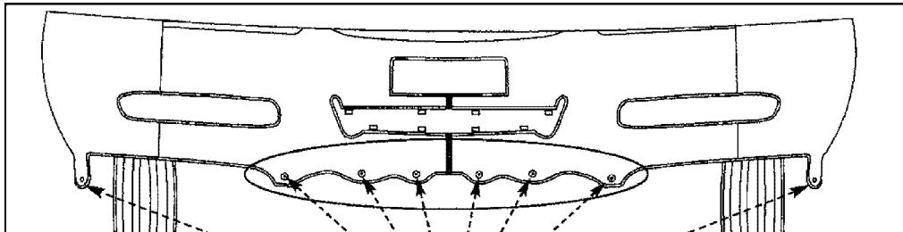
Remove the existing hardware. Insert screws (SS #1) into holes and tighten. Then close the snaps.
