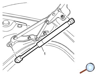
Note: To remove the struts, use a flat blade screwdriver to lift the clip to a 45° angle then rotate the strut off the ball stud.
