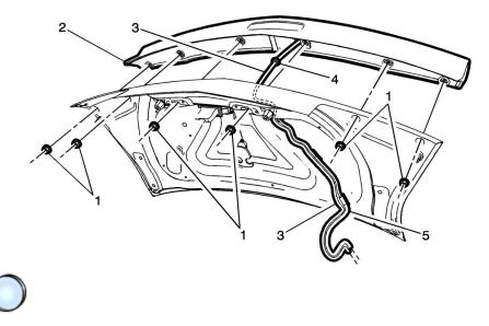
Note: Make sure tape pull tabs are exposed from underside of spoiler.
