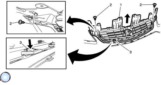
Remove the upper grille (1) from the rear of the fascia by first removing the two retaining screws (2). Release the fascia grille retaining clips (3) (12 places). Carefully pull the grille out from the fascia.
